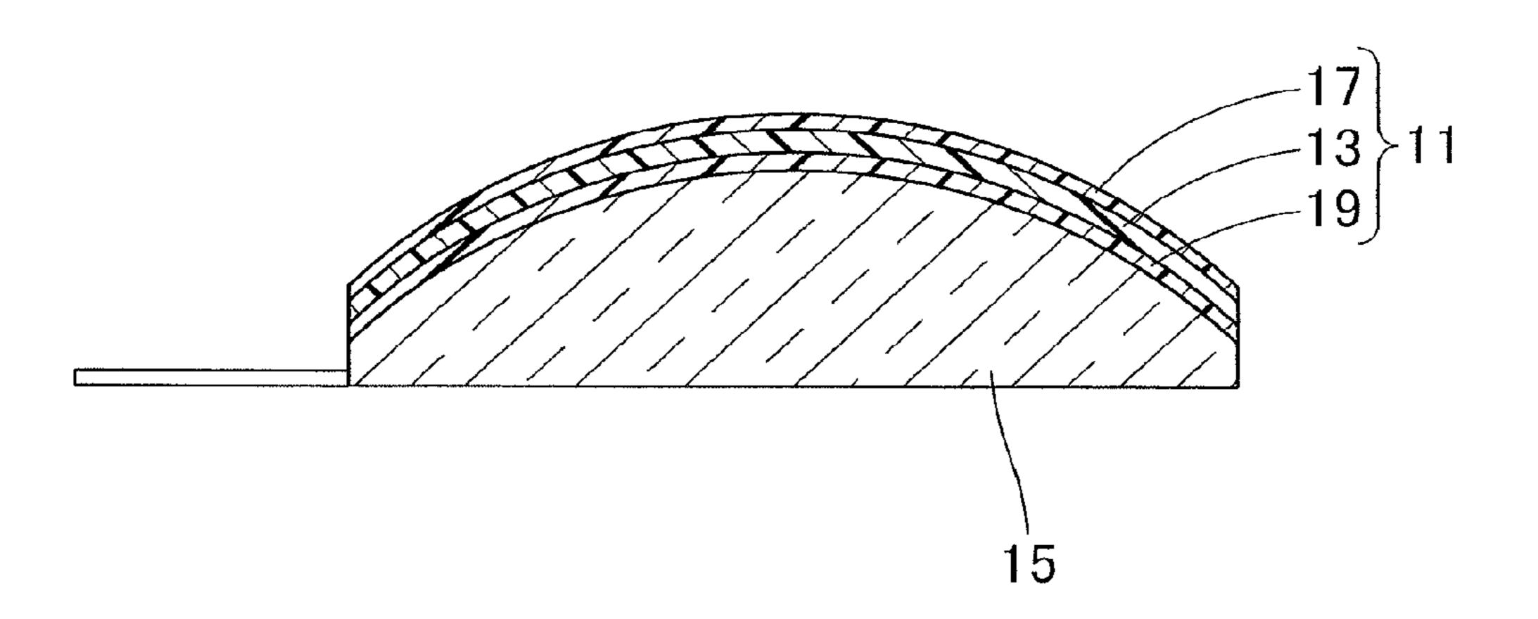
casting method with retardation (Re)≤50 nm. The transparent films for the first and second protective layers are respectively formed from an acylcellulose-based film and a polyamide-based film.
