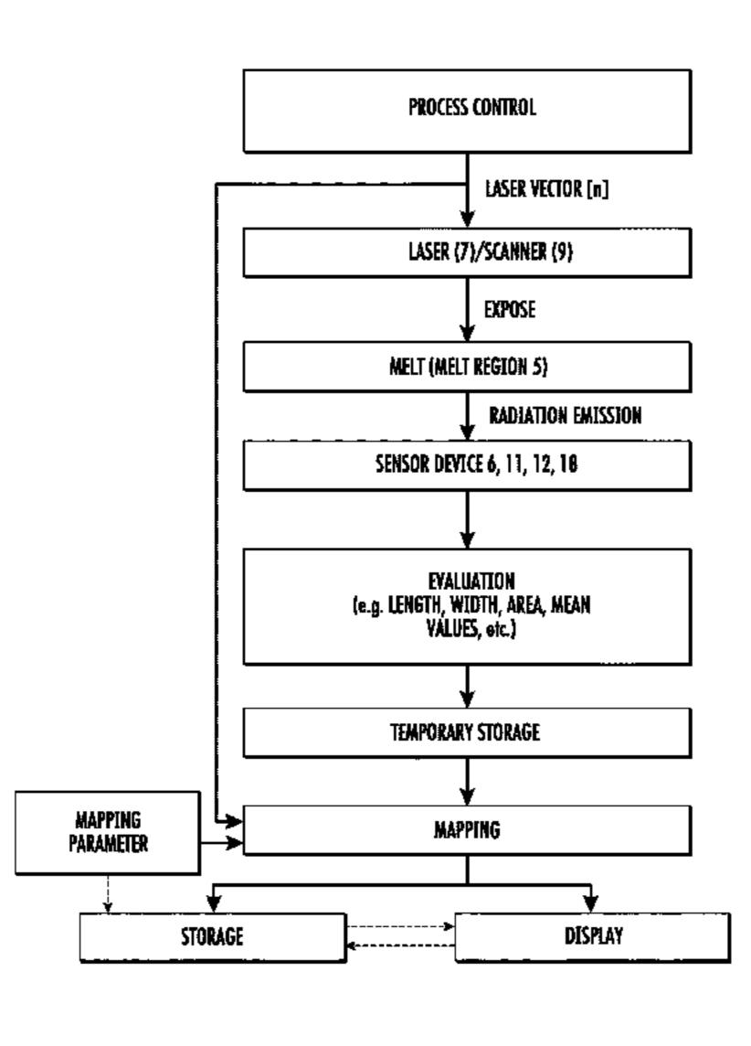
evaluate the component quality. The sensor values detected in order to evaluate the component quality are stored together with the coordinate values that locate the sensor values in the component and are displayed by means of a visualization unit in two- and/or multi-dimensional representation with respect to the detection location of the sensor values in the component.
