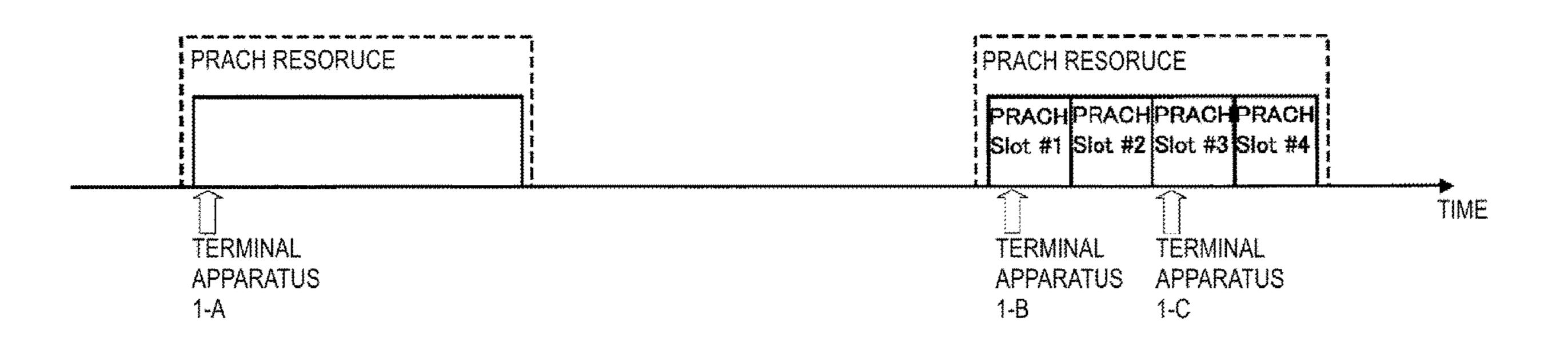
control information is used to configure a subframe number of a second uplink subframe in which transmission of the random access preamble is allowed and a symbol number of an uplink symbol in the second uplink subframe.
