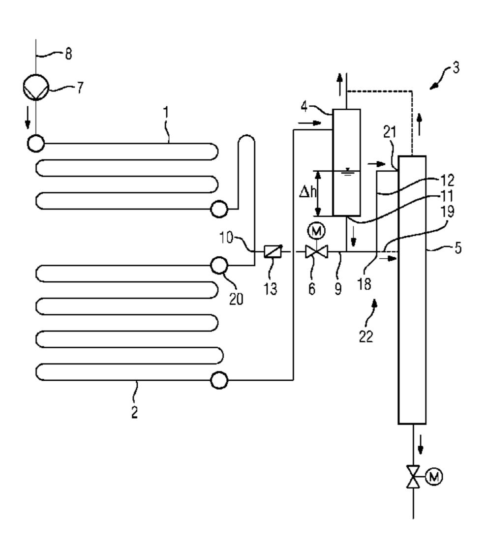
separation system. A corresponding device is for starting a vertical forced-flow steam generator according to the method.
