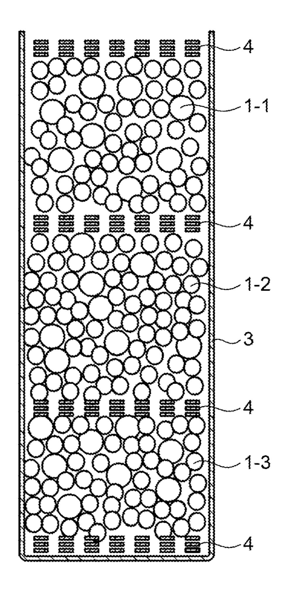
RARE EARTH REGENERATOR MATERIAL PARTICLE, RARE EARTH REGENERATOR MATERIAL PARTICLE GROUP, AND COLD HEAD, SUPERCONDUCTING MAGNET, EXAMINATION APPARATUS, AND CRYOPUMP USING THE SAME
