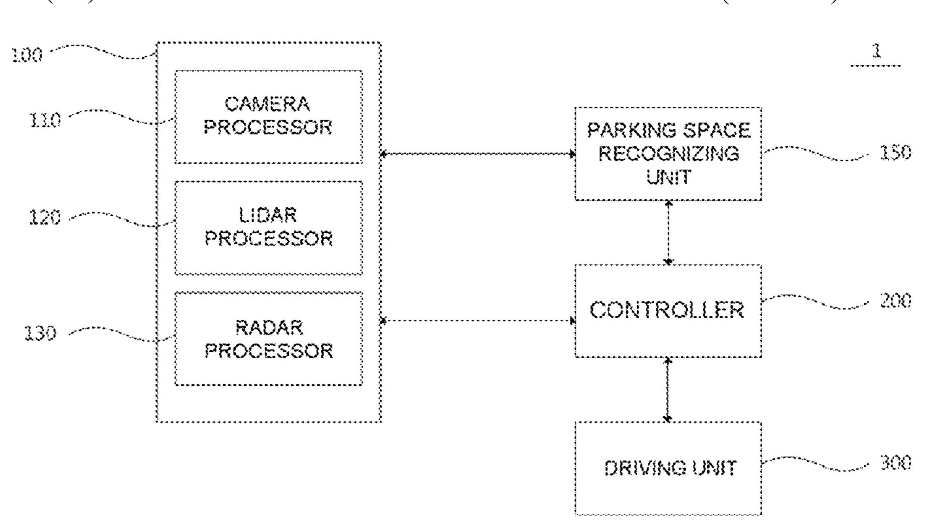
spaced distances and the external images and comparing the consecutive external images with the spaced distances using an image recognition technology to recognize parking areas. A controller calculates a moving path between a current position of the subject vehicle and an optimal parking area and operates the subject vehicle based on the moving path.
