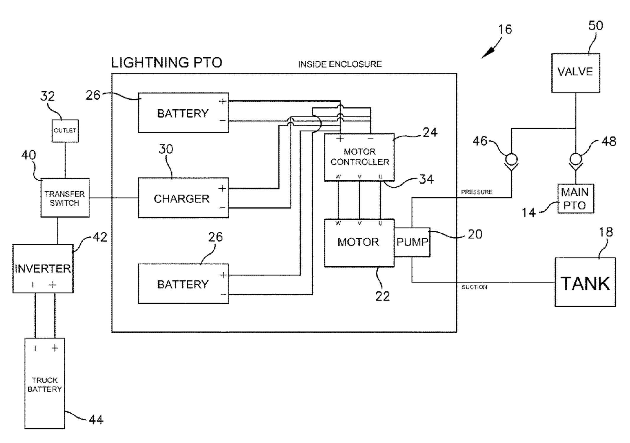
The system also includes a system interlock rendering inoperable the electric power-take-off system when the internal combustion engine is in operation and a motor controller in communication with the motor for controlling the power output of the motor. The system also includes a charging unit for charging of the battery and a data management system operable to collect data.
