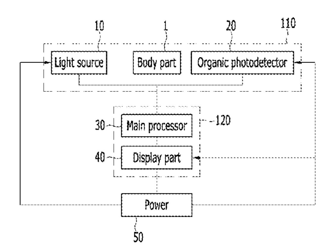
(and/or alternatively predetermined) range being transmitted through the body part. The detector is configured to determine biomedical information of the body part based on an amount of the light sensed by the organic photodetector.
