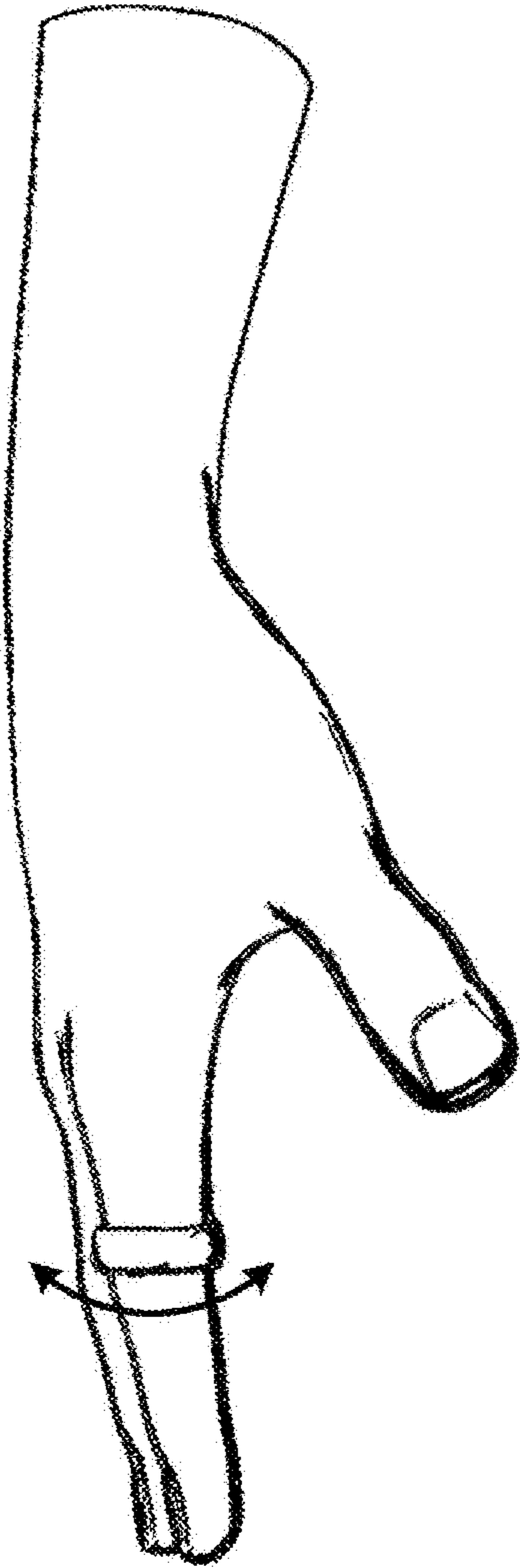
Rotation about x axis (pitch) (Output of acceleration (x axis) of -9.8 to 9.8)
