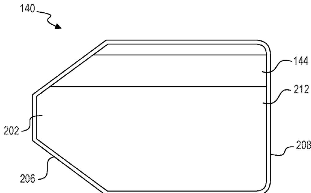
component and the generally planar second card component may be configured such that one forms a container and the other forms a lid configured to close the container.
