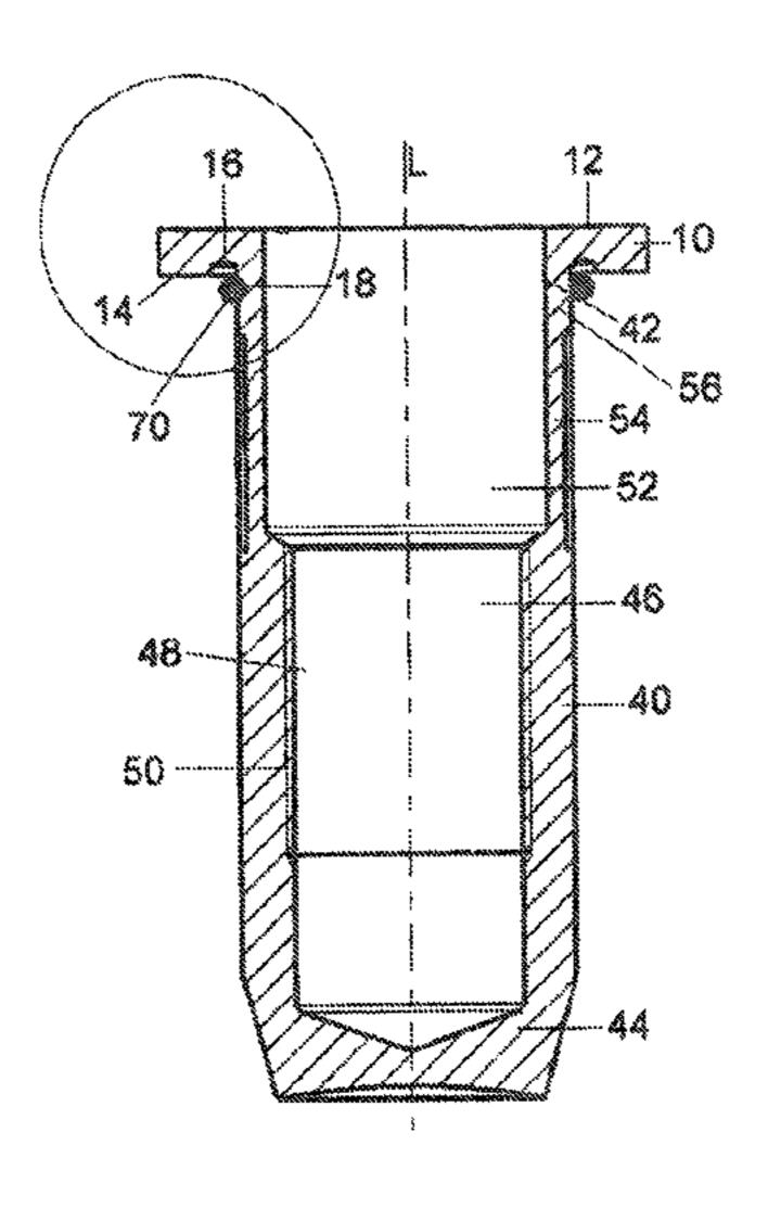
tially around the shank, is arranged adjacent to the underside of the head, and retains the sealing ring in a preloaded position before mounting the blind rivet insert.
