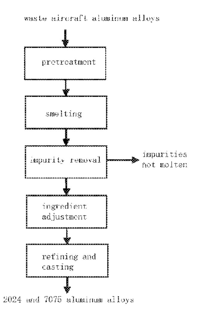
aluminum pop-top cans to adjust the ingredients, the waste aircraft aluminum alloys would be recycled at a lower cost without downgrading. The present invention has some advantages, such as low cost, and applicability for industrial production, as well as prominent economic benefit.
