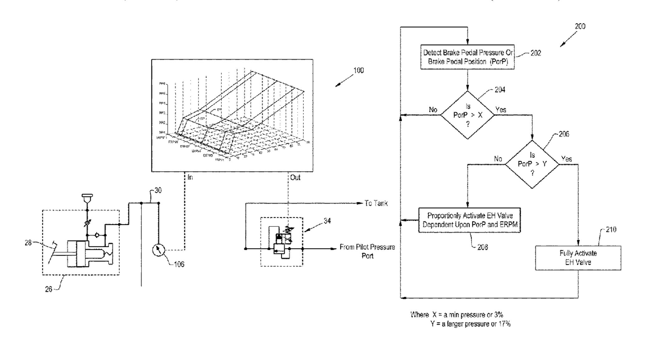
operator. A controller receives the signal and a speed of the engine. The controller controls the electrohydraulic valve dependent upon the signal and the engine speed so that the inching starting point is unchanged regardless of the speed of the engine.
