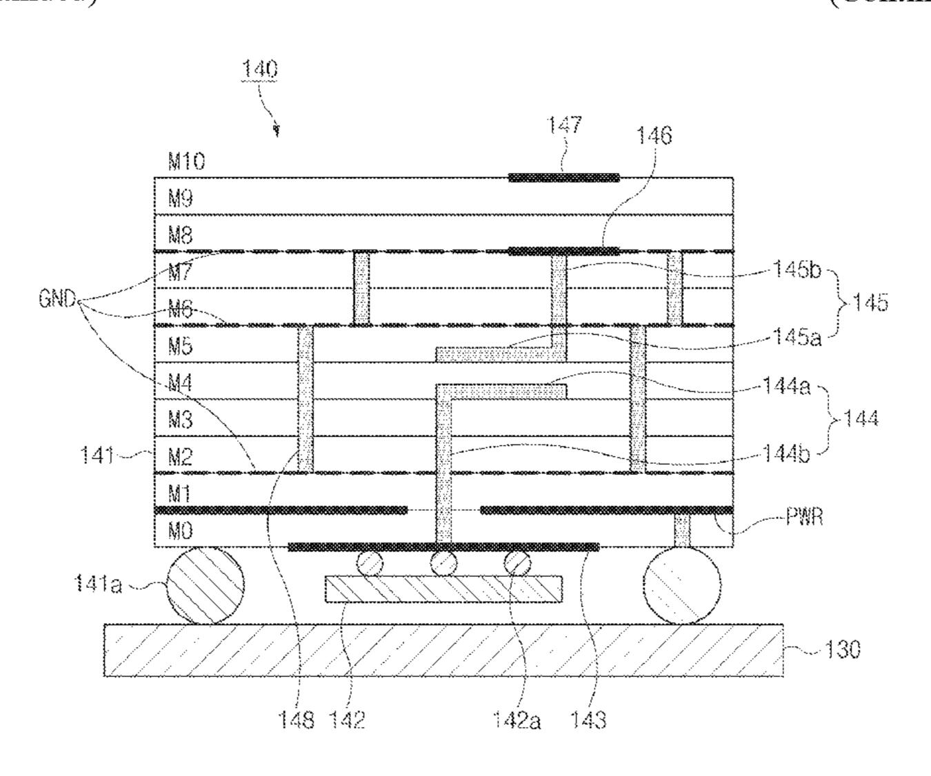
first end and the second end, a second electrical path having a third end electrically connected with the conductive plate and a fourth end floated, the second electrical path including a second portion between the third end and the fourth end.
