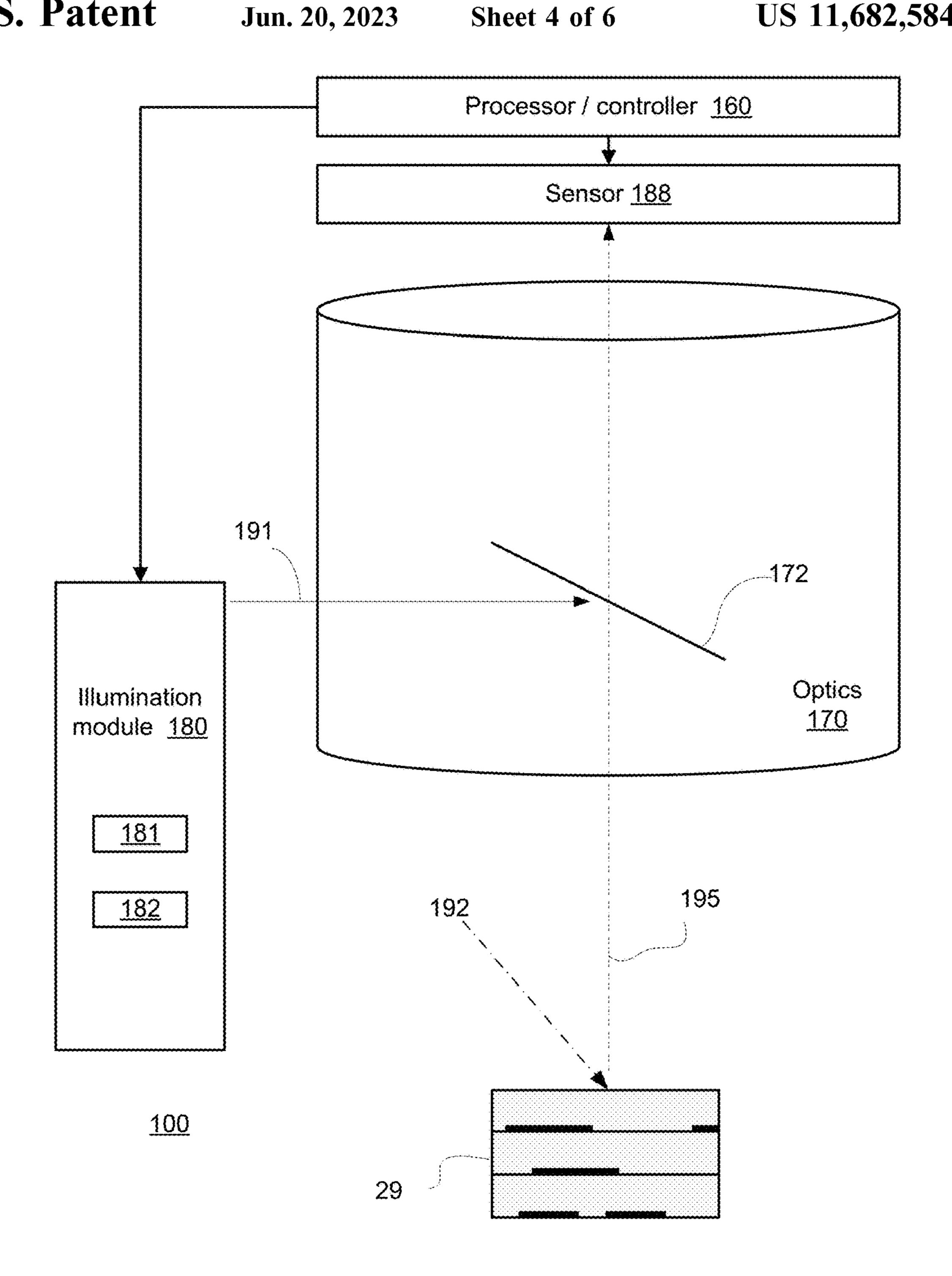
Optimizing the light spectrum to allow adequate contrast between the inspected top RDL layer to the background. 105
