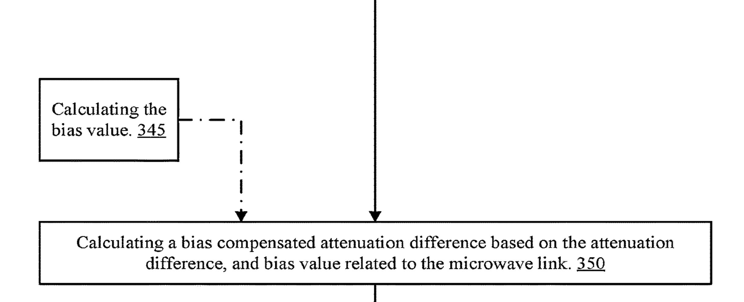
Calculating the rain attribute based on the bias compensated attenuation difference. 360
