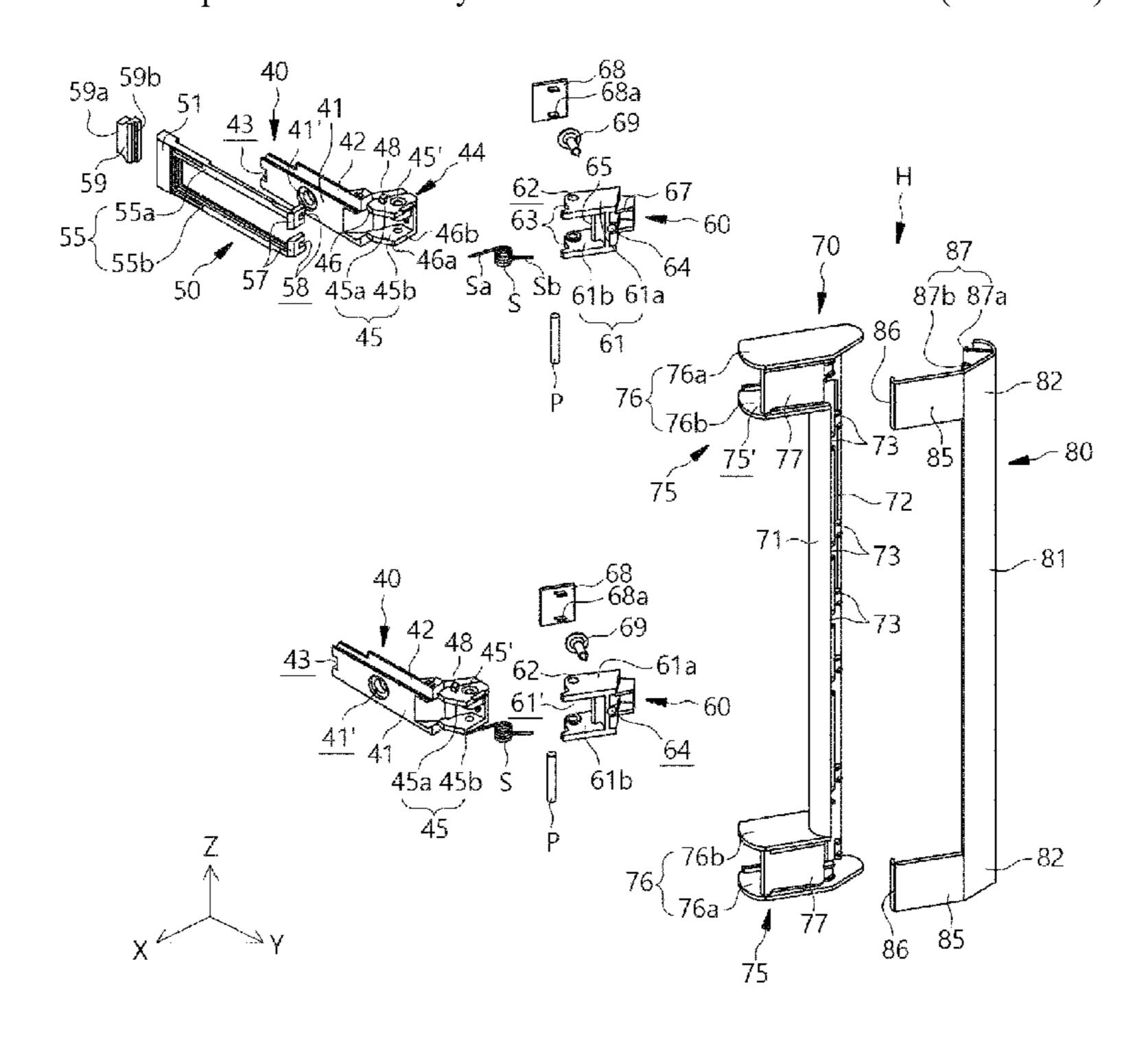
handle cover and configured to push a push rod while the driving arm rotates with the handle body. The driving arm is made of metal.
