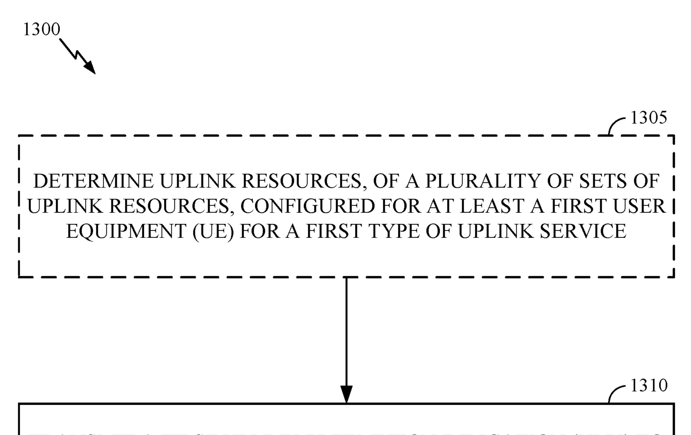
TRANSMIT A FIRST UPLINK PREEMPTION INDICATION (ULPI) TO A USER EQUIPMENT (UE) IN A FIRST ULPI MONITORING PERIOD INDICATING, FOR A FIRST PLURALITY OF SETS OF RESOURCES, WHETHER THE RESOURCES ARE PREEMPTED, WHEREIN A TIME DURATION OF THE PLURALITY OF SETS OF UPLINK RESOURCES IS LONGER THAN A CONFIGURED ULPI MONITORING PERIODICITY FOR THE UE
