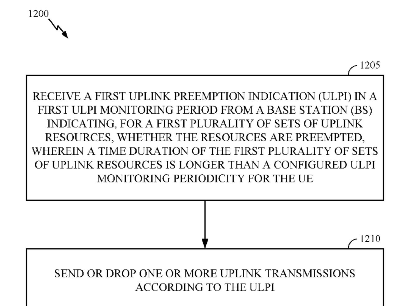
or drops the one or more uplink transmissions according to the ULPI. A time duration of the plurality of sets of uplink resources can be longer than a configured ULPI monitoring periodicity.
