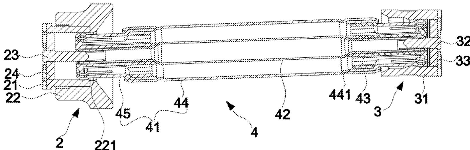
outer circumferential surface. Two ends of the third outer conductor are respectively electrically connected to the first and second outer conductors.
