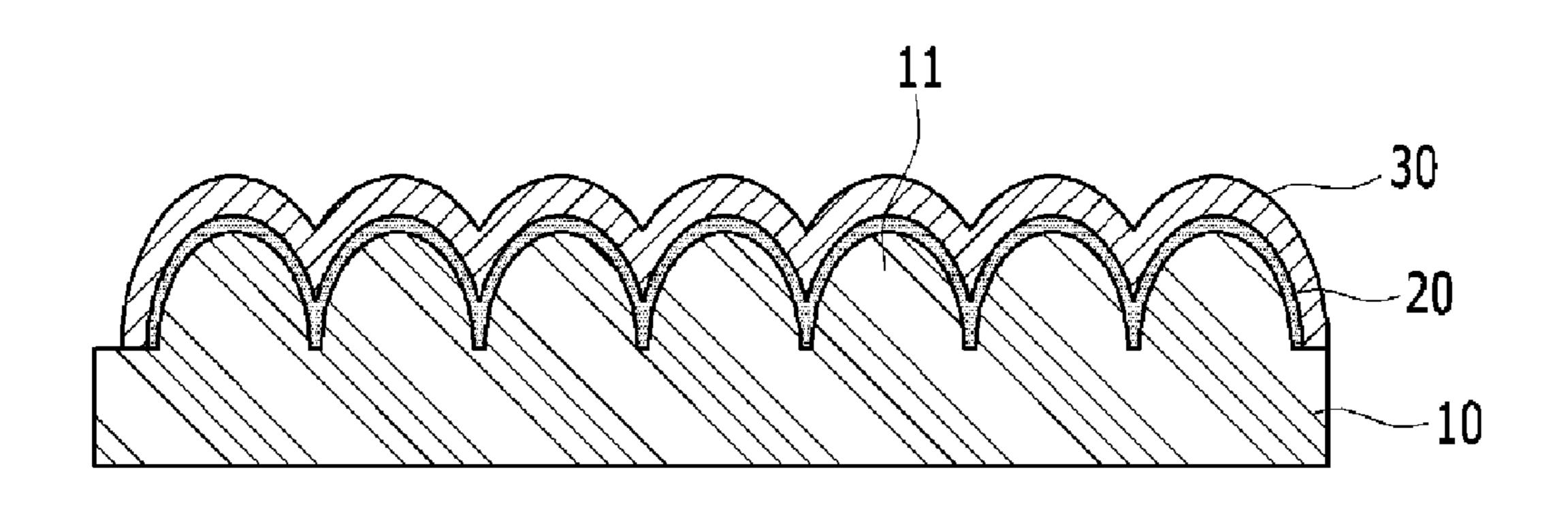
and an active material layer, thereby improving processability during manufacture of the electrode and assembling the battery.
