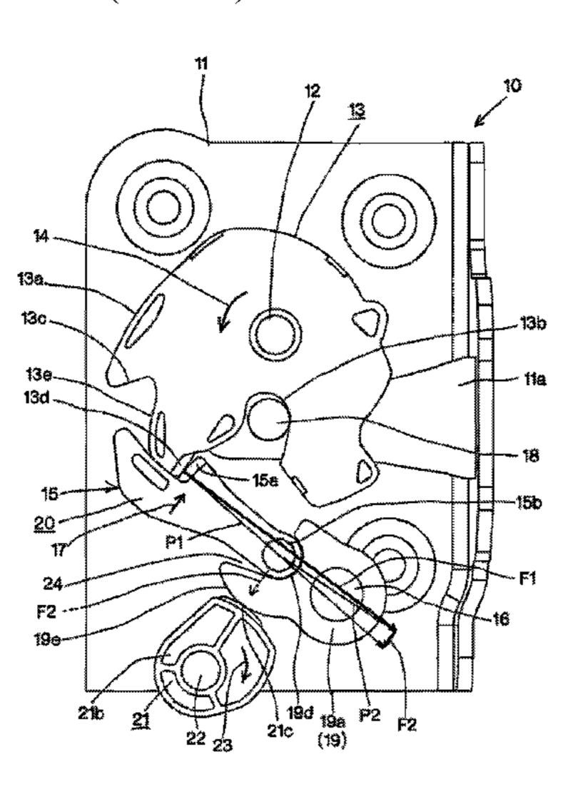
the latch releasing position by the release component force; a ratchet restraint that is arranged on a side of the ratchet member and that can be moved about a pin between a block position and a release position.
