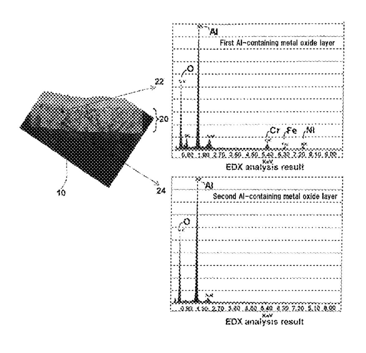
atomic % ratio of Al/(Cr+Ni+Si+Fe), and having a thickness that is at least one fifth of a thickness of the barrier layer.
