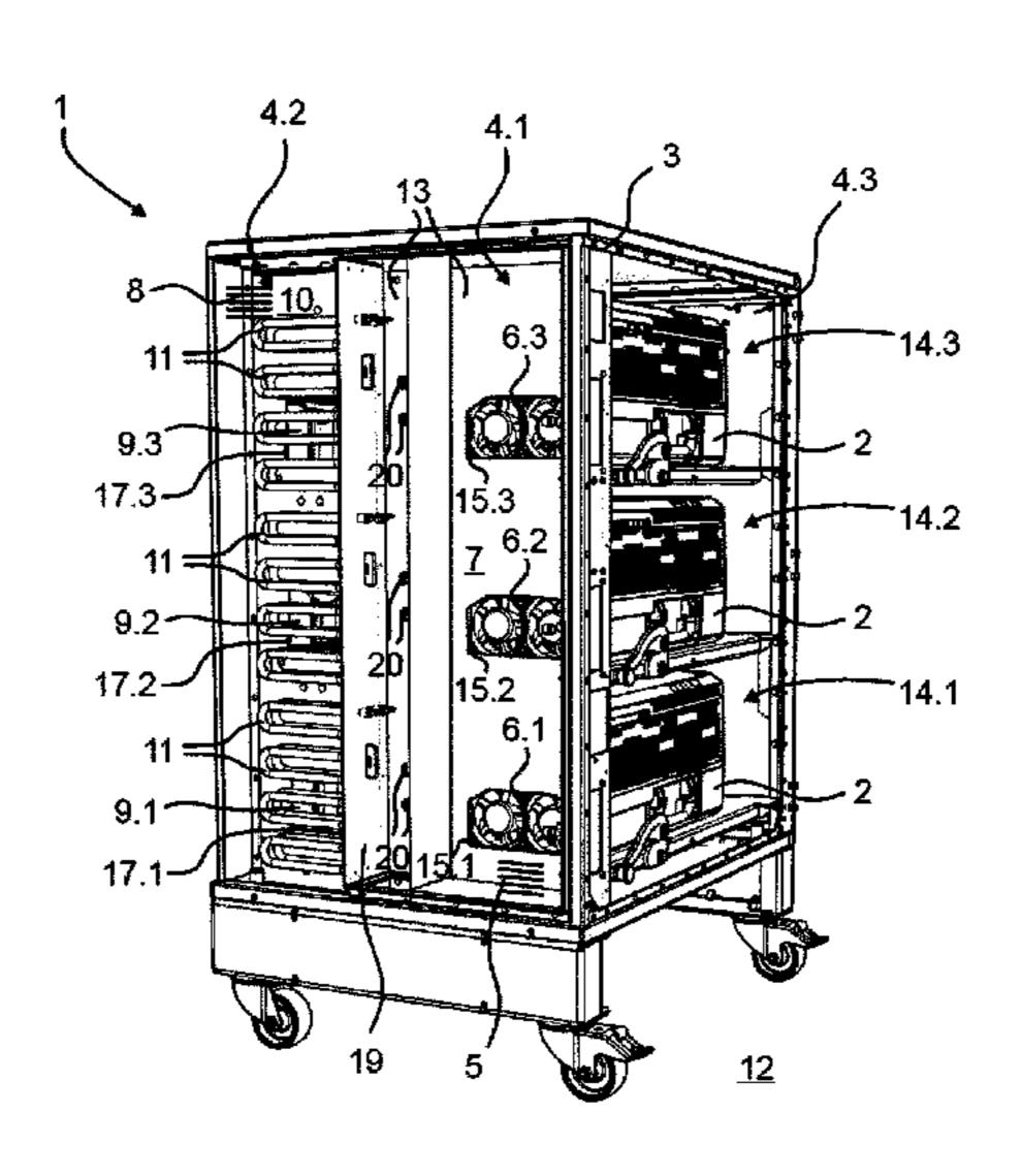
compartment is in the form of a rack with at least one drawer, wherein each drawer is designed to receive an insertable control device.
