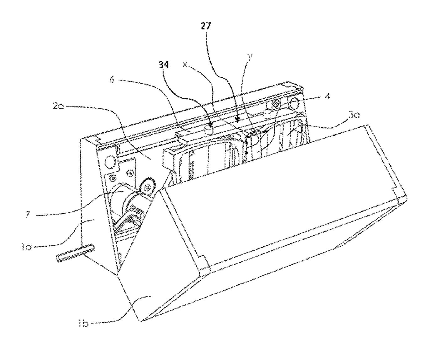
shaped cleaning elements relative to each other substantially parallel to the opposing faces of the glasses while rubbing or wiping them clean.
