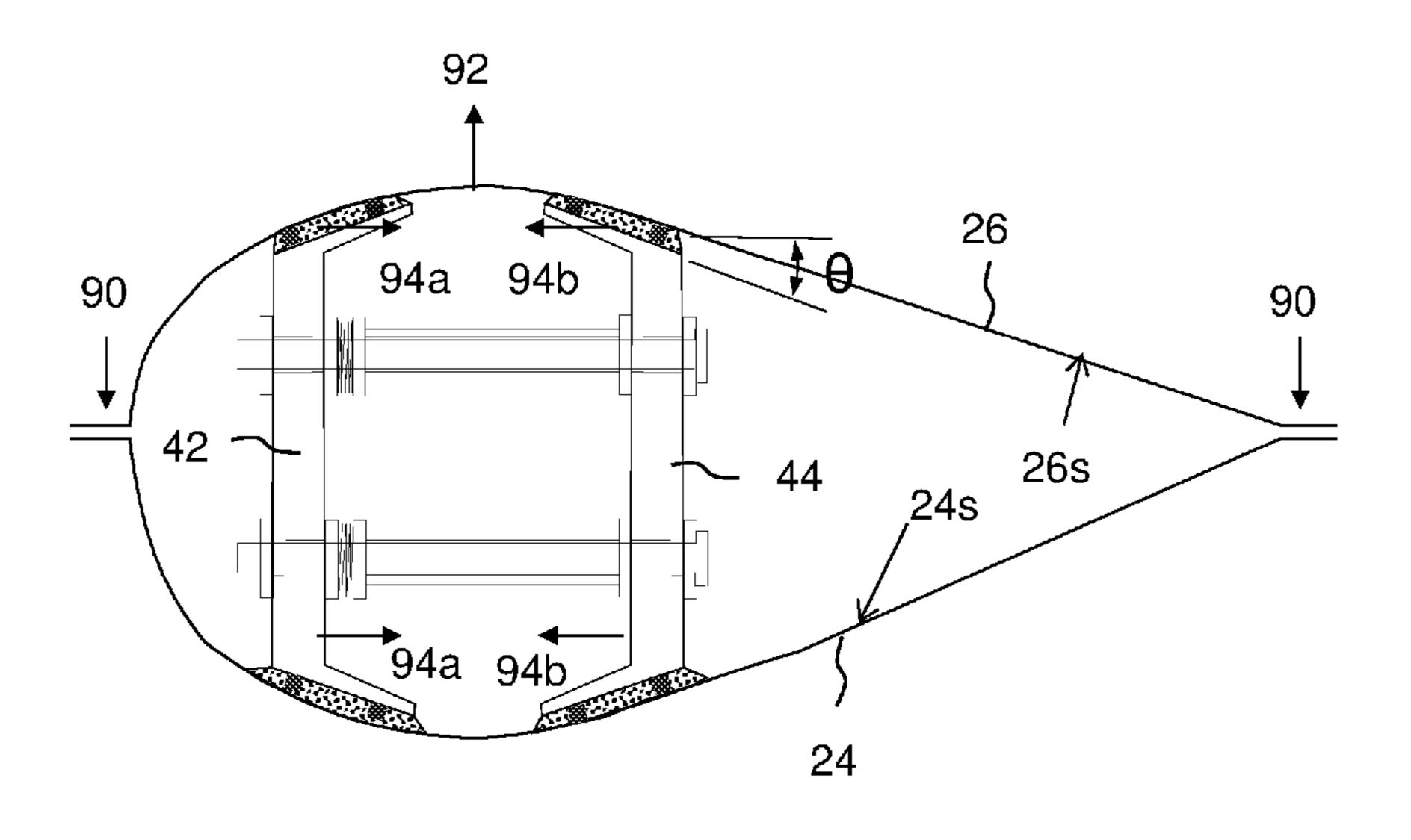
shear web. The first shear web and the second shear web are placed in the lower shell part and the upper shell part is mounted.
