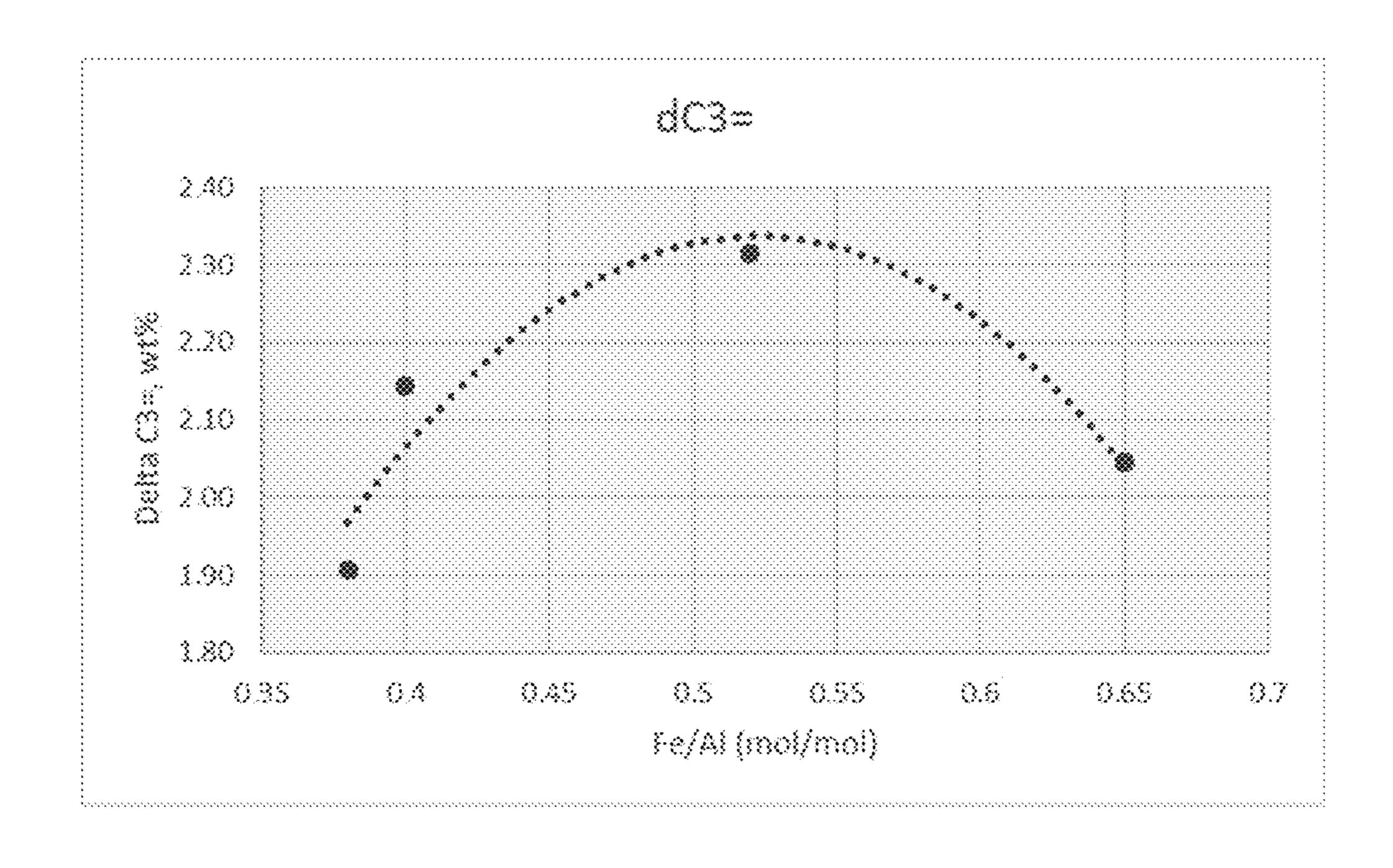
FIG. 2: Propylene make vs P(Fe + Al) molar ratio
