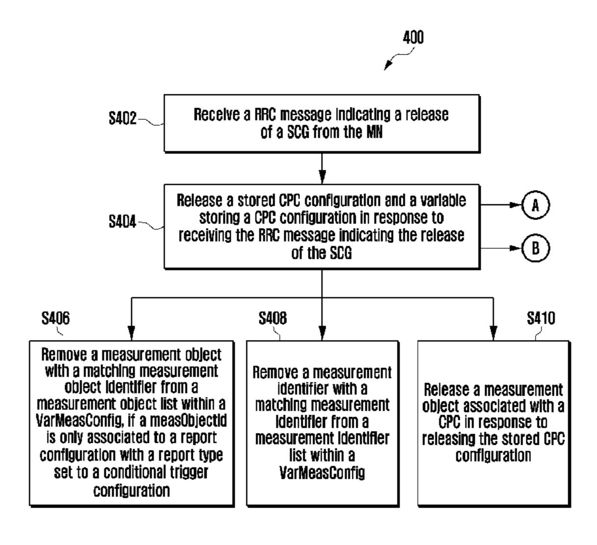
releasing a secondary cell group of the second base station is received from the first base station, releasing the stored CPC configuration.
