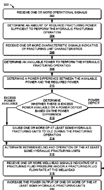
difference is indicative of a power deficit, increasing a power output of at least one of the hydraulic fracturing units.
