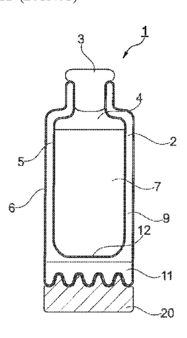
state, in which the working medium (11) is in the solid state and is in contact with the outer wall (6), and is not in contact with the inner wall (5), and a thermally conductive state, in which at least some of the working medium (11) is in the liquid state and has expanded and is in thermally conductive contact both with the outer wall (6) and with the inner wall (5). The invention also provides a method for controlling the temperature of food or of a beverage in a portable hand-held device.
