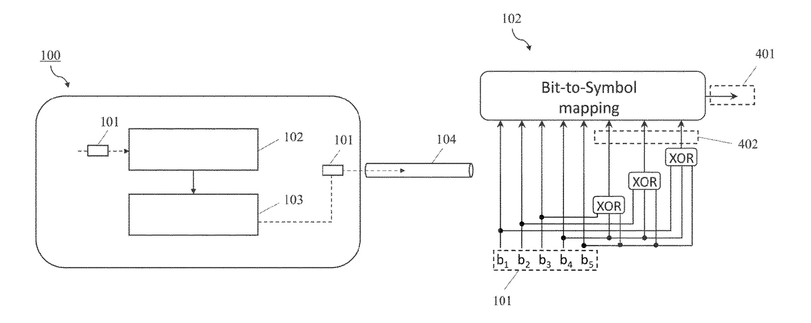
polarizations of an optical carrier. Symbols in consecutive transmission time slots have non-identical polarization states.
