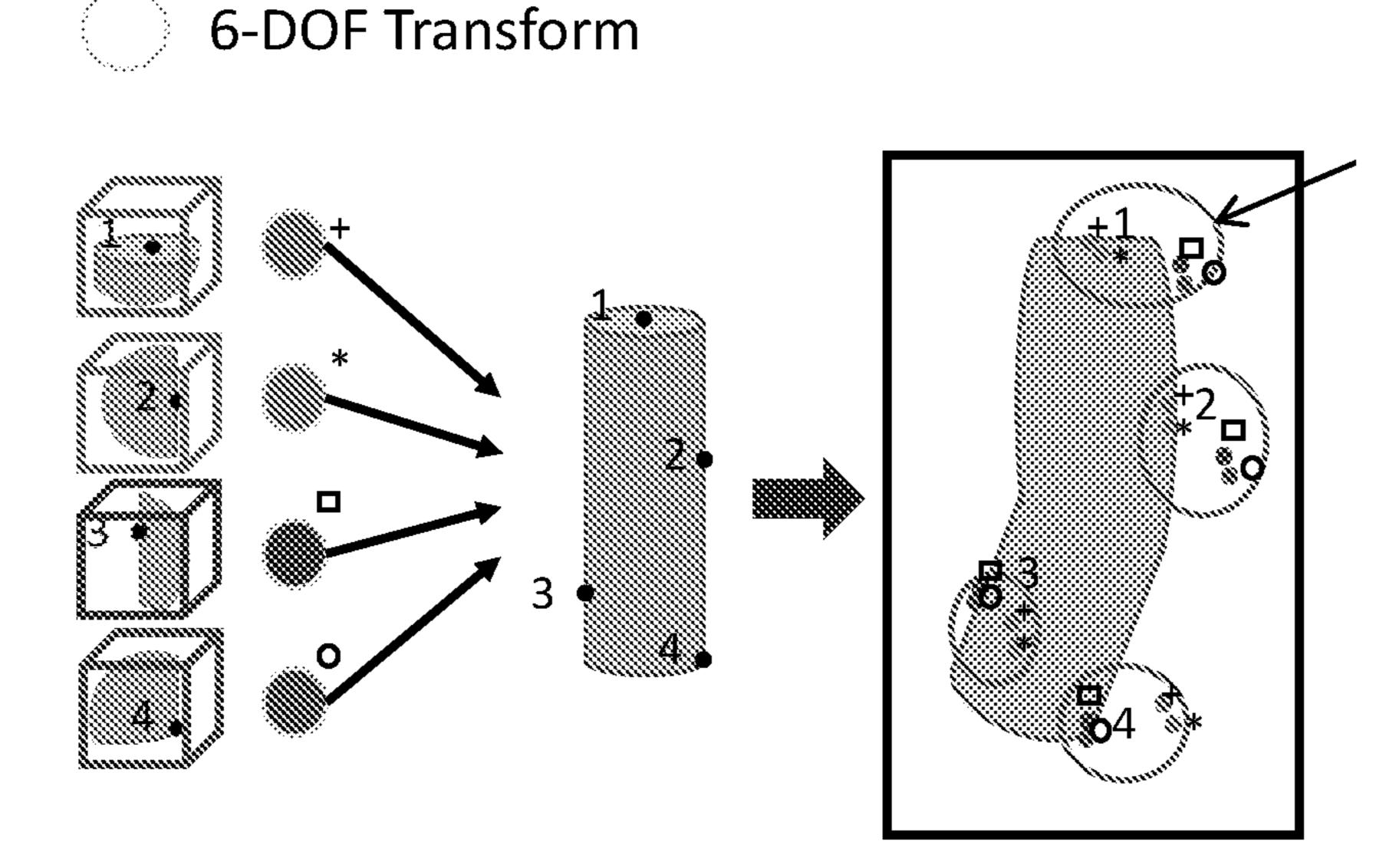
Point cloud of annotation 1's projected location using each of the four 6-DOF outputs. Note that, as expected, the projection using the 6-DOF transform for annotation 2 projects to a similar location as annotation 1.
