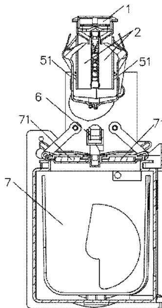
receiving lateral wings are butted in a space between the ice making assembly and the water collecting tank to form a closure space with an opening facing the ice making assembly, and a water outlet communicating with the water collecting tank is constructed on one side of the closure space. The present application may solve the problems of condensed water dripping out and water splashing outward during ice making.
