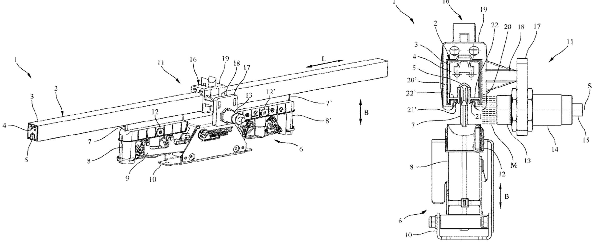
by the sensor being designed for contactless and/or contacting detection of the measurement indicator, and by means of a brushgear system having a device of this kind, and also a method of this kind in which the sensor detects the measurement indicator becoming closer to the sensor contactlessly and/or contactingly and, when a threshold value for a predetermined wear of the sliding contact is exceeded, issues a warning signal.
