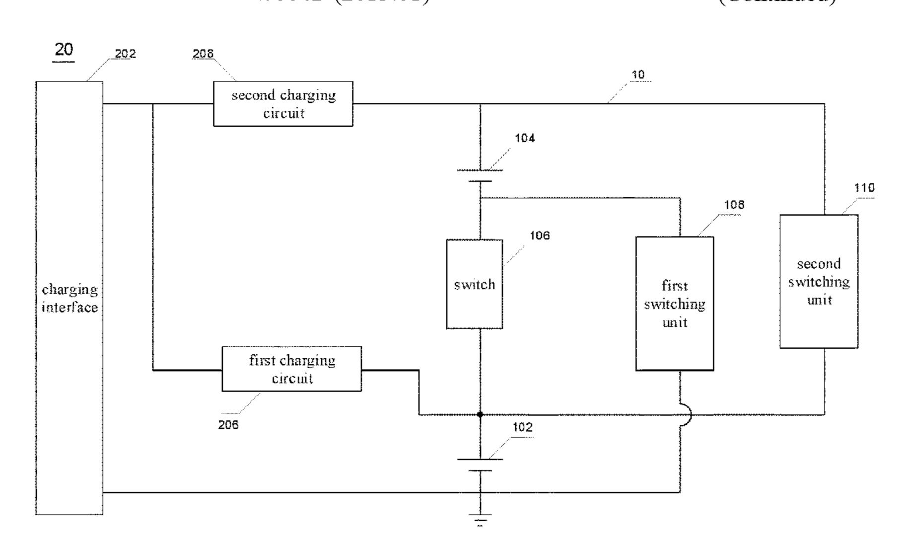
the output voltage and current on both ends of the first and second cells coupled in series, or directly apply the output voltage and current on both ends of the first and second cells coupled in parallel.
