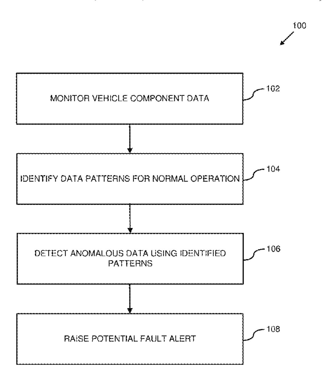
FIG. 1 100 MONITOR VEHICLE COMPONENT DATA -104IDENTIFY DATA PATTERNS FOR NORMAL OPERATION 106 DETECT ANOMALOUS DATA USING IDENTIFIED PATTERNS RAISE POTENTIAL FAULT ALERT
