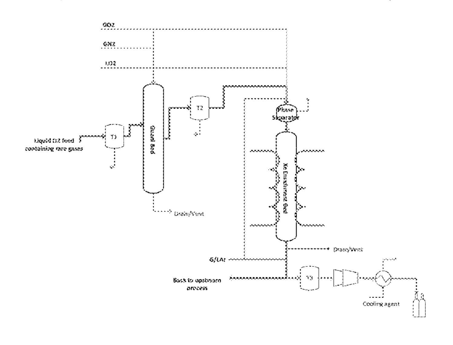
displacing the adsorbed oxygen and other residues with argon, prior to regeneration, along with indirect heating of the bed, enables production of a high purity product ≥40 vol % xenon from the adsorption bed and further enables safely heating without any purge gas and ease for downstream product collection, even in cases where hydrocarbons are co-present in the feed stream.
