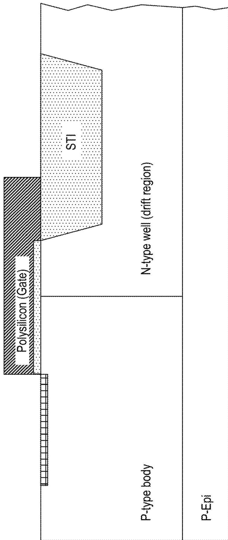
Shallow Arsenic implantation. The gate poly enables self-alignment of the implant.
