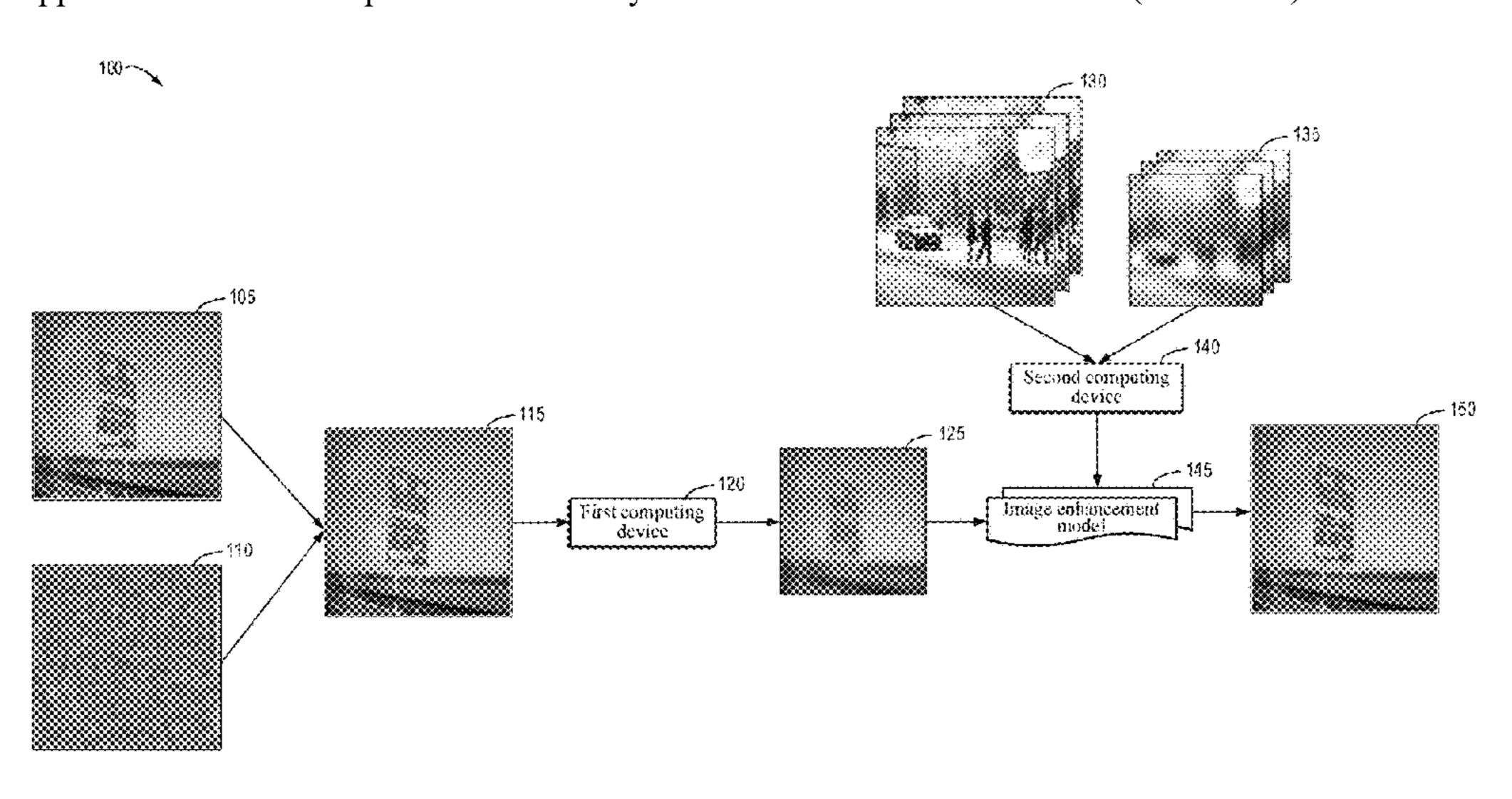
sample image; and generating a target image by processing the intermediate image using the image enhancement model, the target image having an image quality higher than the intermediate image.
