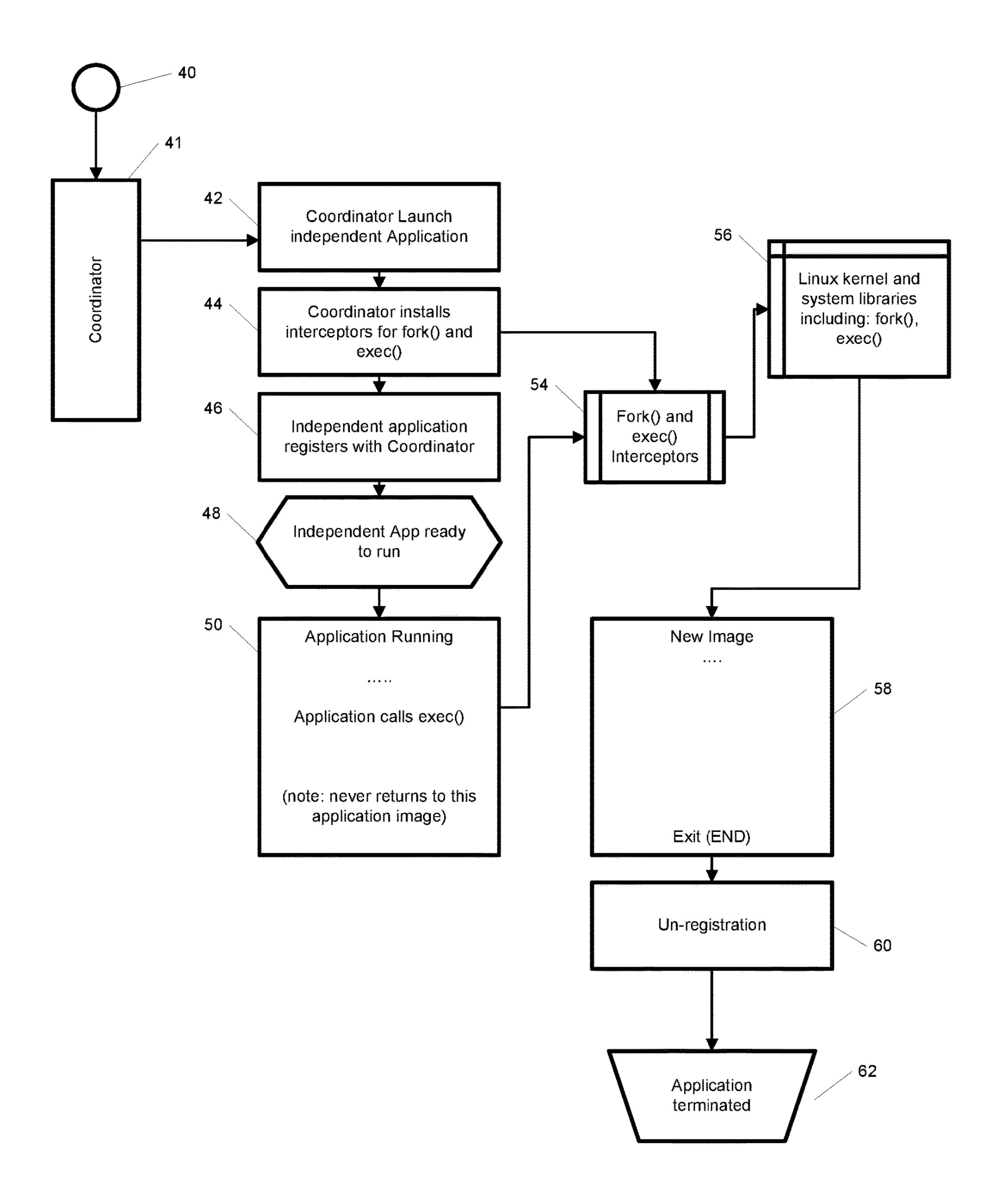
Fig.2 –Core operation of exec()
