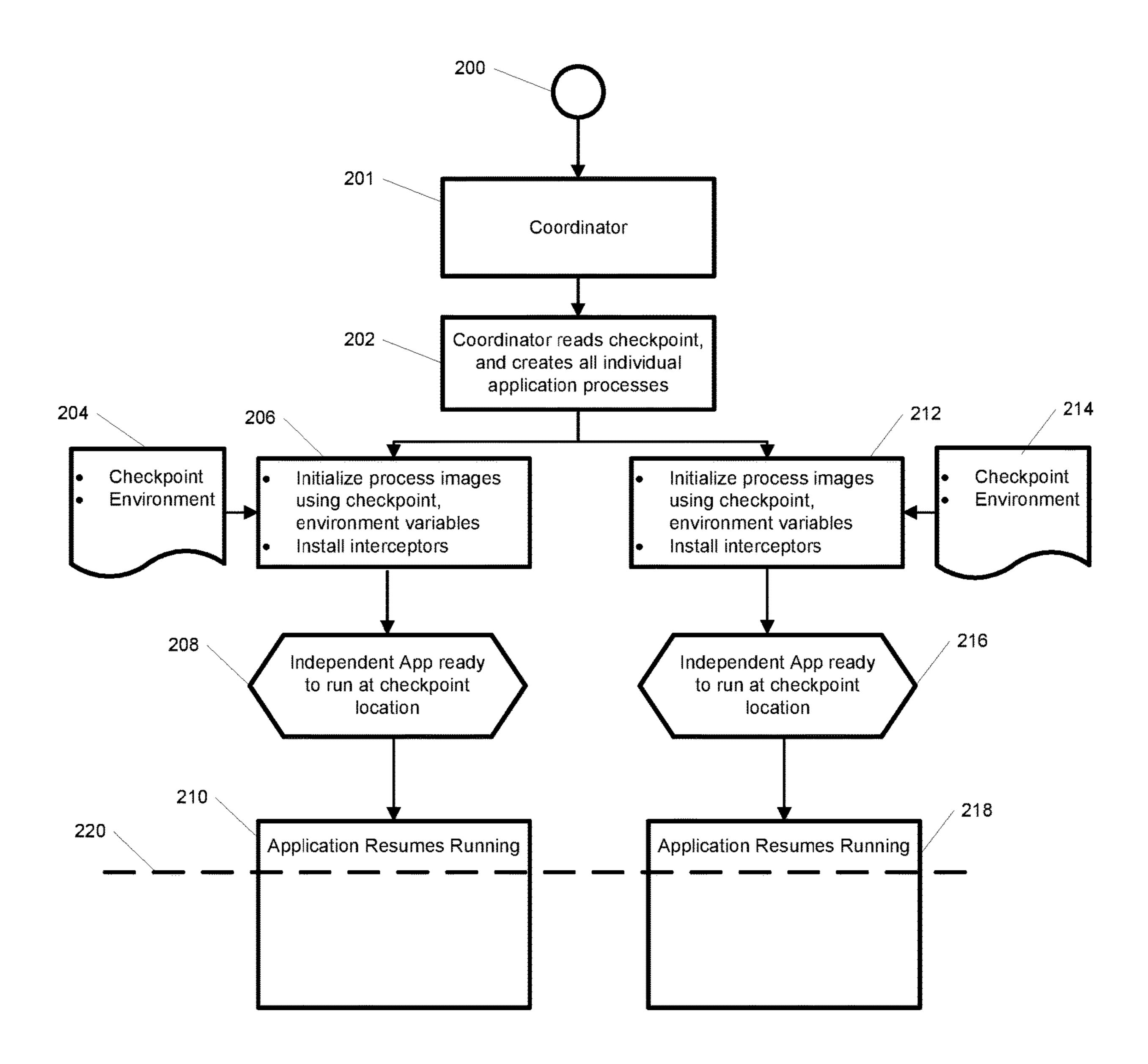
Fig.7 – Restoring an application group from a checkpoint
