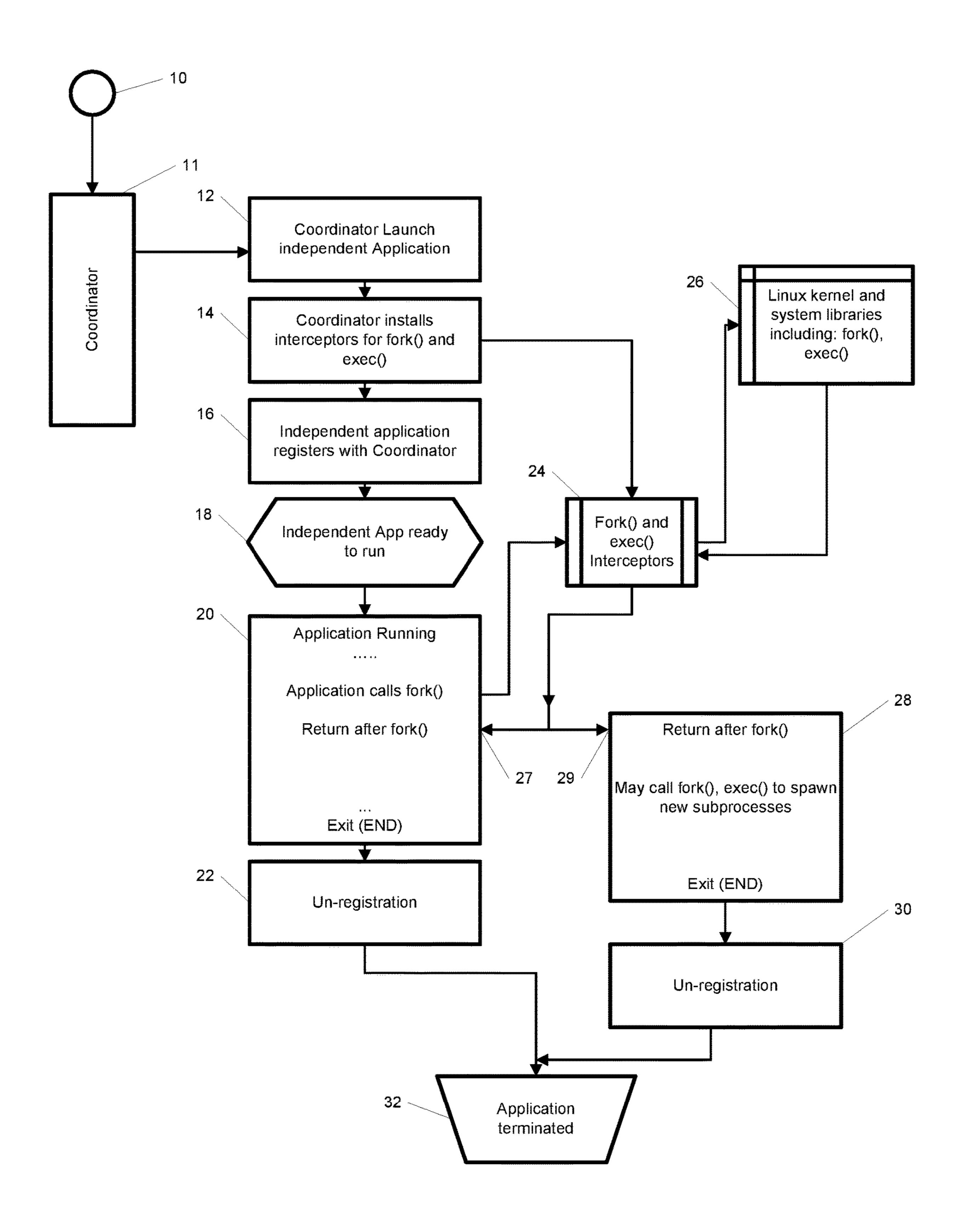
Fig. 1 – Core operation of fork()
