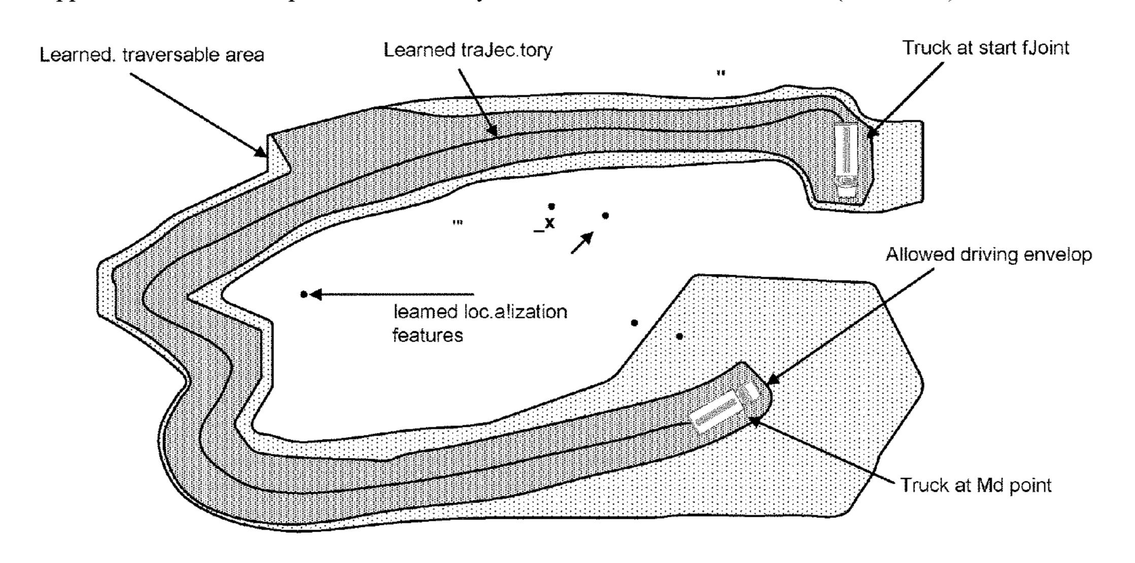
the truck automatically learn the route using features in the environment to localize. In future runs, the truck is able to automatically follow the learned route.
