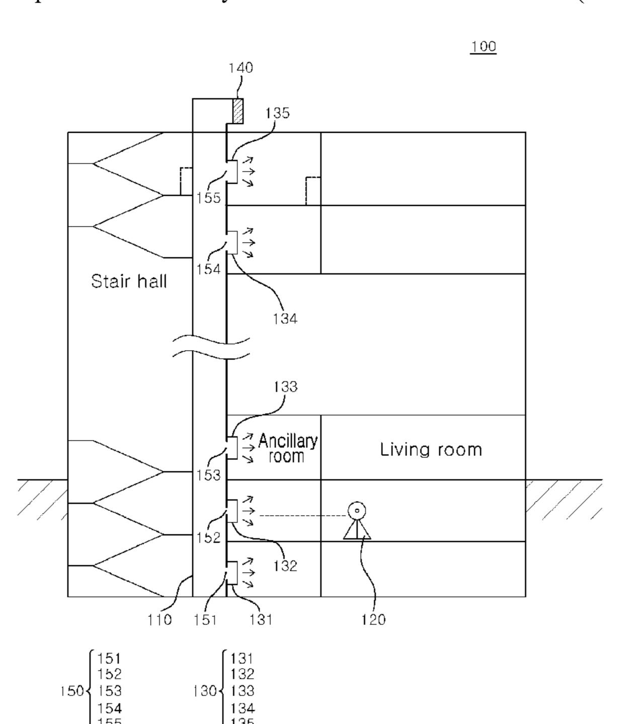
a plurality of automatic differential pressure dampers installed in a plurality of ancillary rooms provided on the plurality of floors, respectively, to be adjacent to the plurality of openings. Opening areas of the plurality of openings increase as locations of the plurality of openings become farther away from a point, at which air is supplied to the supply air duct by the blower.
