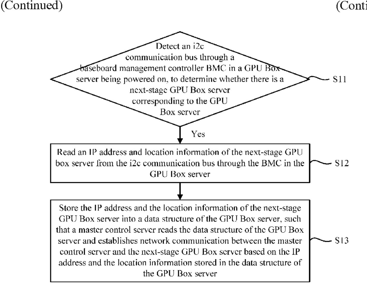
GPU Box server; and storing the IP address and the location information of the next-stage GPU Box server into a data structure of the GPU Box server so that a master control server reads the data structure of the GPU Box server, and establishing network communication with the next-stage GPU Box server according to the IP address and the location information stored in the data structure.
