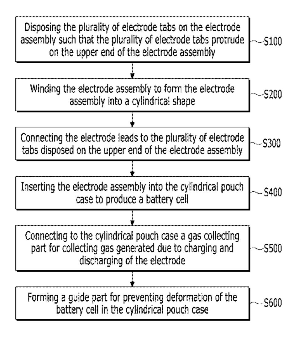
part for collecting gas generated due to charging and discharging of the electrode; and forming a guide part for preventing deformation of the battery cell in the cylindrical pouch case.
