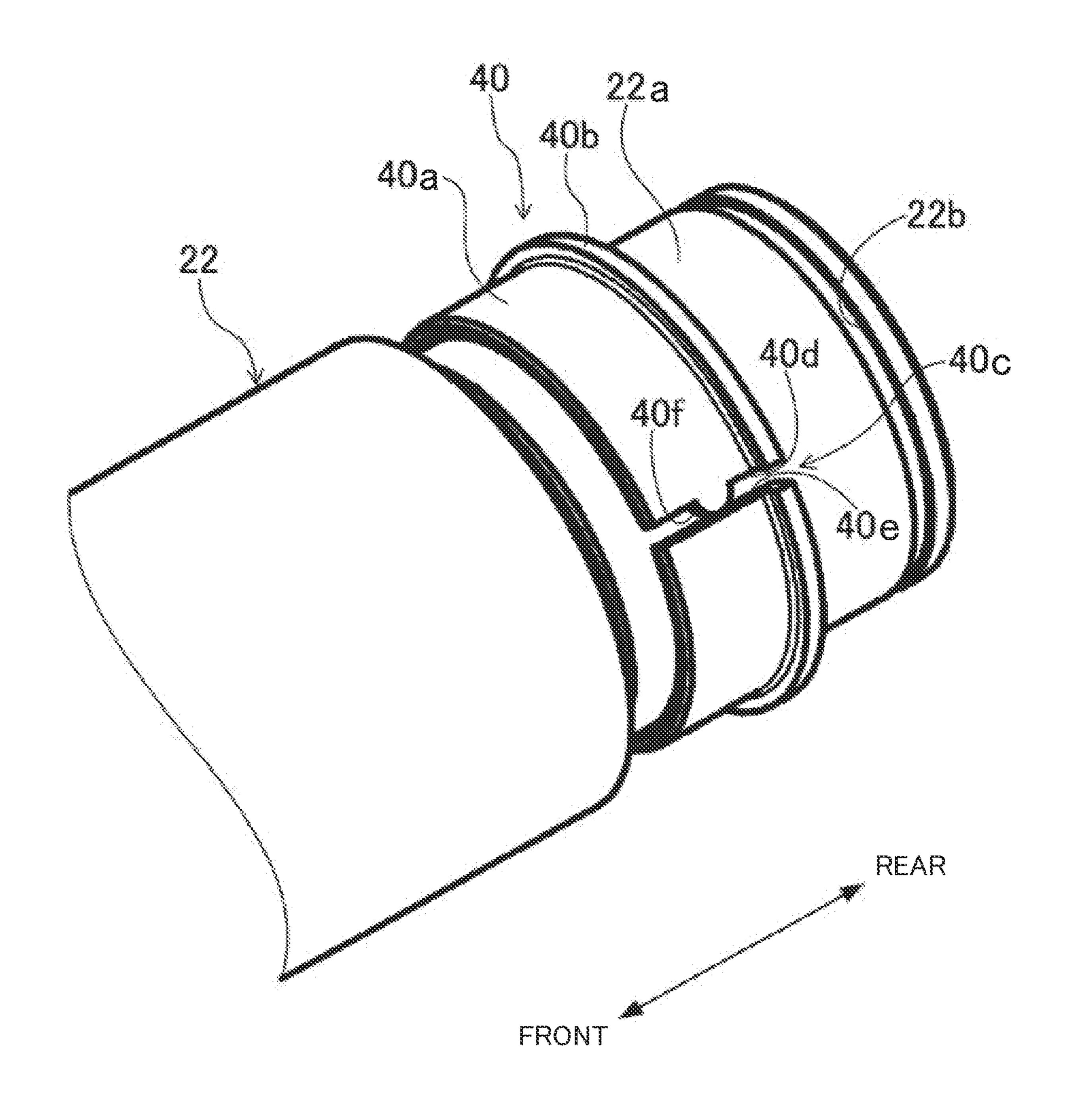
FIXING DEVICE INCLUDING INSULATING MEMBER WITH SLIT FORMED WITH PROJECTION PROJECTING FROM ONE END SURFACE TOWARD THE OTHER OF SLIT, AND IMAGE FORMING APPARATUS WITH FIXING DEVICE
