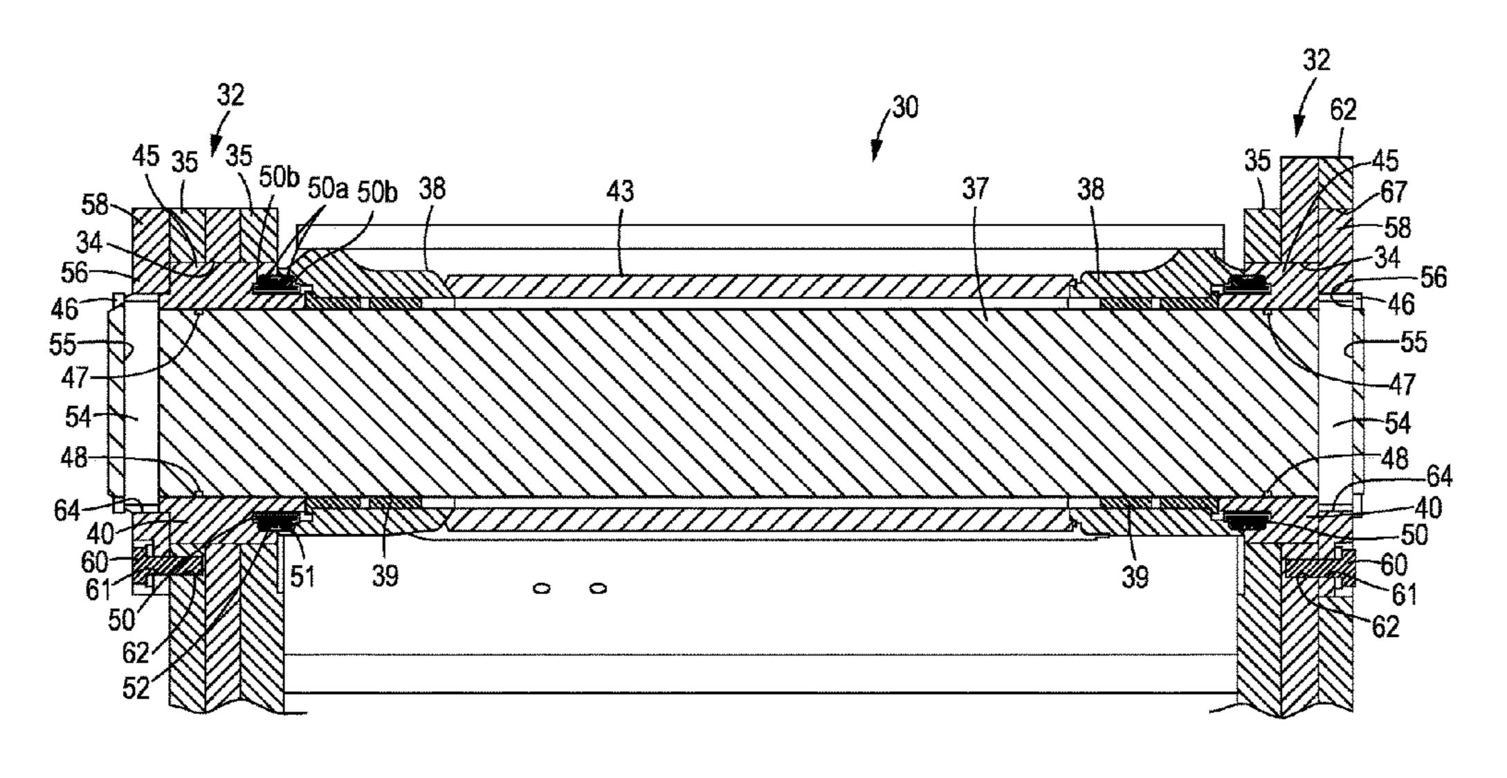
portion. The bearing device comprises a bracket having an opening for mounting the collar.
