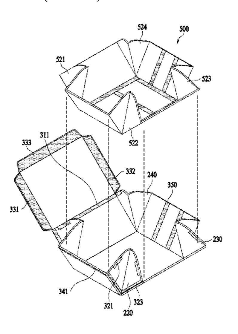
bottom portion and to face the sidewall portions of said box portion; and reinforcing joint portions configured to join said reinforcing sidewall portions, to be folded to face itself and to be in close contact with the reinforcing sidewall portions, upon conversion into the box mode, and wherein said reinforcing bottom portion, said reinforcing sidewall portions and reinforcing joint portions form a single plane in the unfolding mode.
