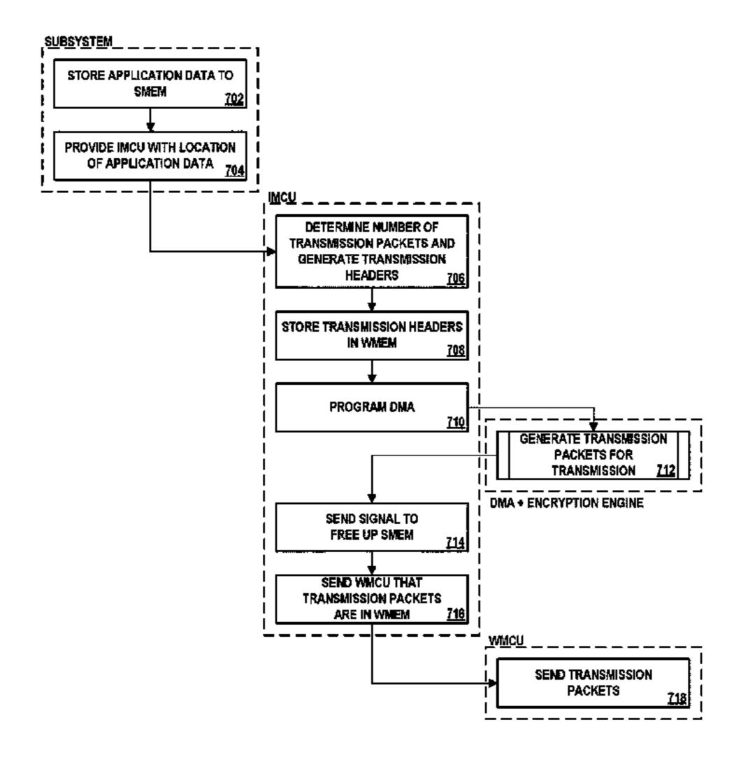
application data packets, and outputs the encrypted application data packets for storage to the first memory.
