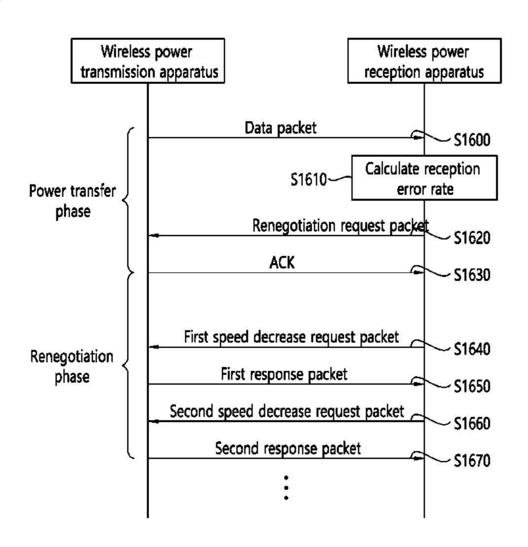
transmission apparatus; and changing the communication speed of the wireless power transmission apparatus on the basis of the first request packet, and transmitting, at the changed communication speed, a first response packet in response to the first request packet to the wireless power reception apparatus.
