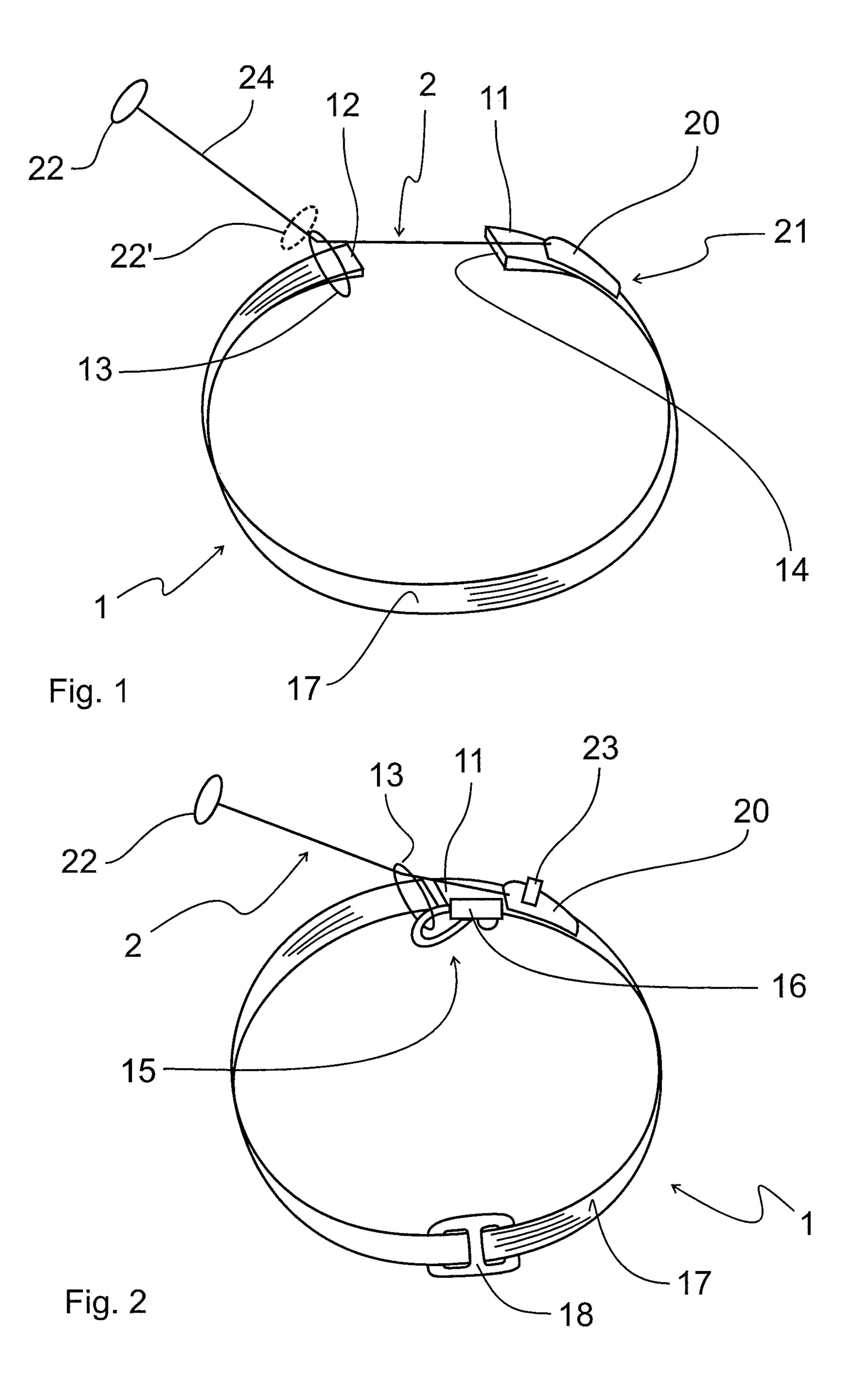
This invention relates to a dog collar-leash combination with a collar and with a leash in a housing, with a rolling and unrolling mechanism, wherein the leash in the housing can 5 be unwound against a spring force and where the outer end
