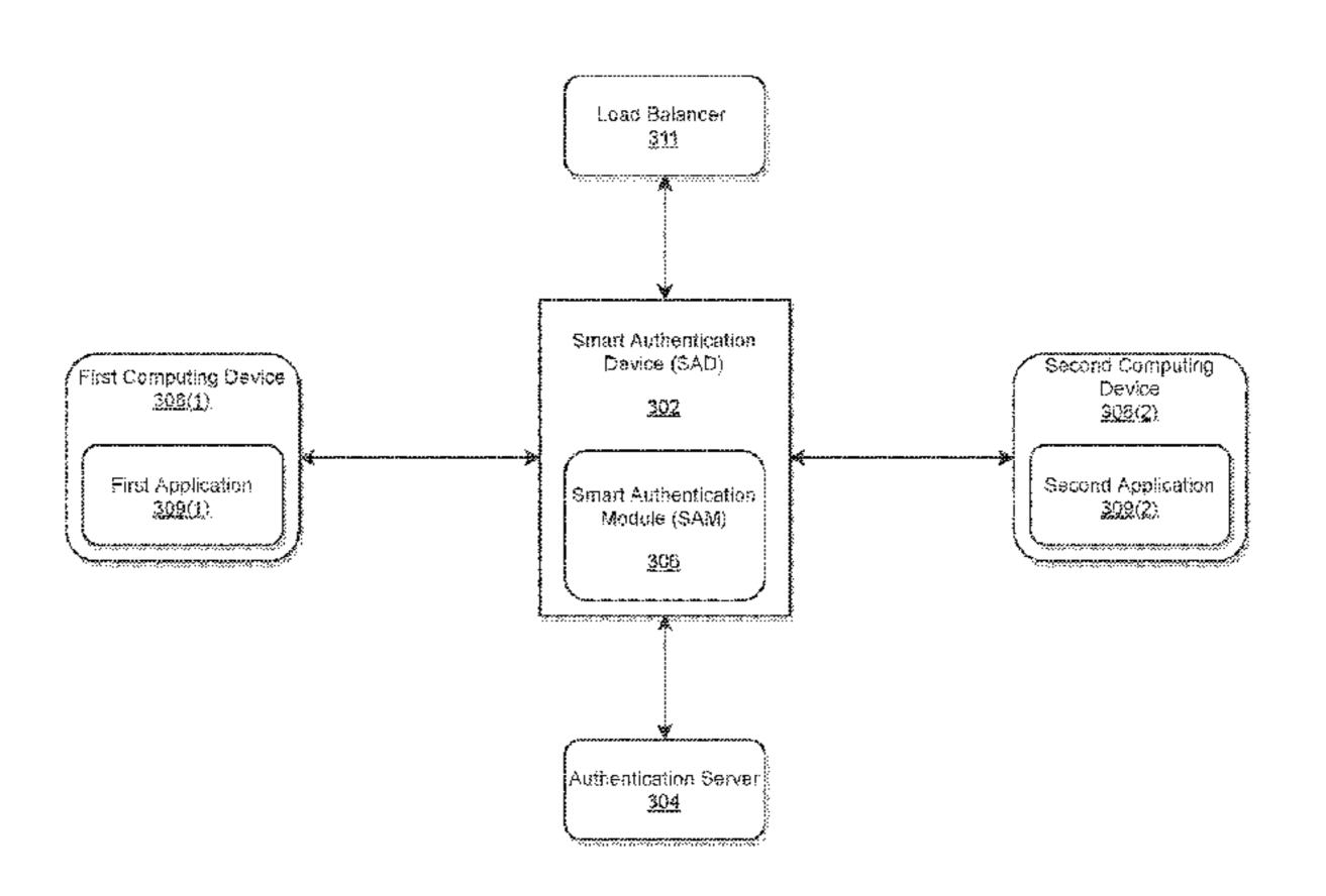
to the second authentication model. The processor transmits a message to the second application and automatically establishes a communication between the first application and the second application in response to receiving the message by the second application.
